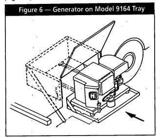
The tray on which the generator rests is hinged, permitting it to swing downward after two side support rails and a center support rail are unbolted.
